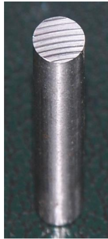
Fig. 1b Cylindrical mild steel C-50 pin
