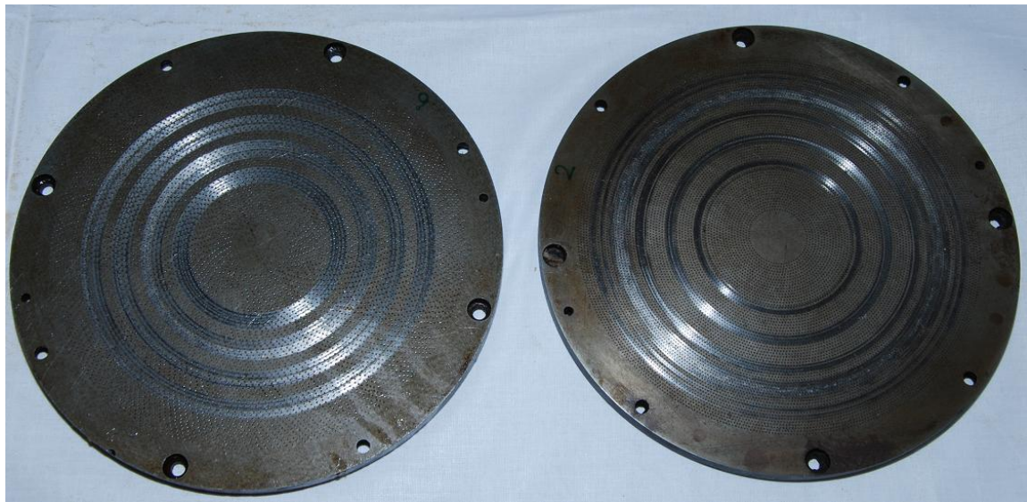
Fig: 4b. Disc with worn track
